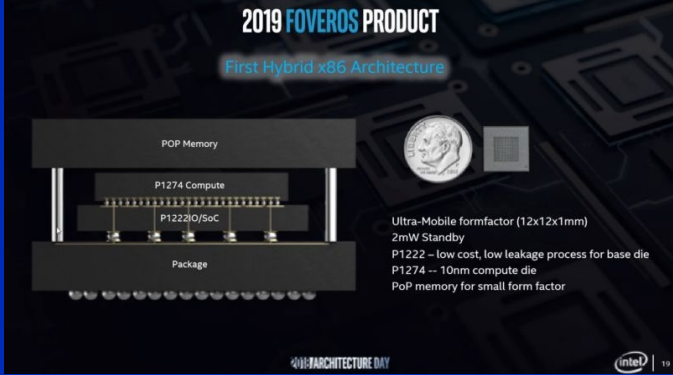
Through Silicon Via (TSV), Intel FOVEROS
